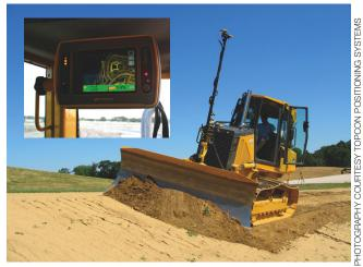
**GPS-CONTROLLED EARTH MOVING** virtually eliminates the need for any grade staking. The on-board control panel, (inset) provides real-time location and grade information.
